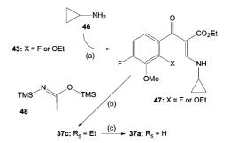
(b) PhMe, rt, 0.5 h; (b) PhMe, reflux, >0.5 h; (c) 32% HCl, EtOH, reflux 5 h.
