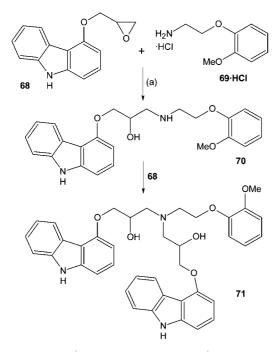
(a) (i)  $K_2CO_3$ ,  $Pr^iOH$ , 83 °C, 5 h; (ii) Filter, distil  $Pr^iOH$ ; (iii) EtOAc, 35 °C, seed; (iv) Centrifuge.
