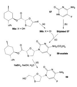
(a) (i) MsOH, DMF, DCM, 8 °C; (ii) 15 °C, 4 h; (iii) Evaporate; (b) (i) HMDS, MsOH, PhMe, reflux, 3 h; (iii) Evaporate; (iii) Et<sub>3</sub>N, DCM, 25 °C; (c) (i) Reflux, 21 h; (ii) Cool, 25 °C, H<sub>2</sub>O; (iii) (CO<sub>2</sub>H)<sub>2</sub>, MeOH, 25 °C, 3 h, filter; (d) (i) KHCO<sub>3</sub>,  $K_2$ HPO<sub>4</sub>, THF, MeOH, H<sub>2</sub>O, <5 °C, 3 h; (ii) 25 °C, 1 h; (iii) 37% HCI to pH 4; (iv) Evaporate.
