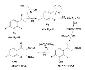
(a) TsOH, PhMe, reflux; (b) (i) Bu<sup>n</sup>Li, THF, -40 °C, 1 h; (ii) B(OMe)<sub>3</sub>, -40 °C, 1 h; (iii) HOAc, -30 °C; (iv) H<sub>2</sub>O, rt, 16 h; (v) H<sub>2</sub>O<sub>2</sub>, rt, 1 h; (c) (MeO)<sub>2</sub>SO<sub>2</sub>, K<sub>2</sub>CO<sub>3</sub>, PhMe, reflux, 1 h; (d) NaH, PhMe, 90 °C, 1 h; (e) PhMe, reflux, 1 h;
