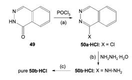
(a) (i)  $POCI_3$ , PhMe, rt; (ii) 65 °C, 3 h; (iii) Aq HCI, EtOAc, rt; (b) (i) EtOH, <5 °C, 24 h; (ii) MeOH, C, rt. 0.5 h, filter; (iii) HCl gas, 0.25 h, filter; (c) (i) MeOH, Et\_3N, 65 °C, filter; (ii) HCl gas, <5 °C, 1 h, filter; (iii) H<sub>2</sub>O, C, EDTA, 80 °C, 0.5 h, filter hot; (iv) MeOH, <5 °C; (v) -20 °C, filter, wash, dry.
