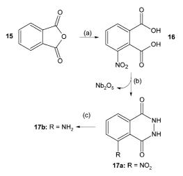
(a)  $HNO_3/H_2SO_4$ ; (b) (i)  $NbCI_5$ , dioxane, rt; (ii) 40% aq  $H_2NNH_2$ , 50 °C, 4 h; (iii) Cool, filter off solids; (iv) Extract with EtOAc, wash, dry; (c) Pd/C,  $H_2$ , dioxane.
