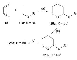
(a) BHT, 135 °C, 16 h; (b) Pd/C, 0.8 MPa H<sub>2</sub>, rt, 2.5 h;
