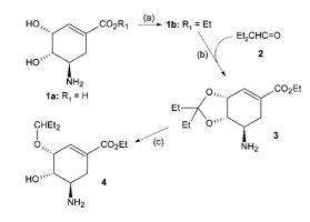
(a) MsOH, EtOH, reflux, 1 h; (b) MsOH, reflux, 2 h; (c) (i) Et<sub>3</sub>SiH, TiCl<sub>4</sub>, DCM, -70 C; (ii) -25 °C, 18 h; (iii) Et<sub>3</sub>SiH, -25 °C, 6 h.
